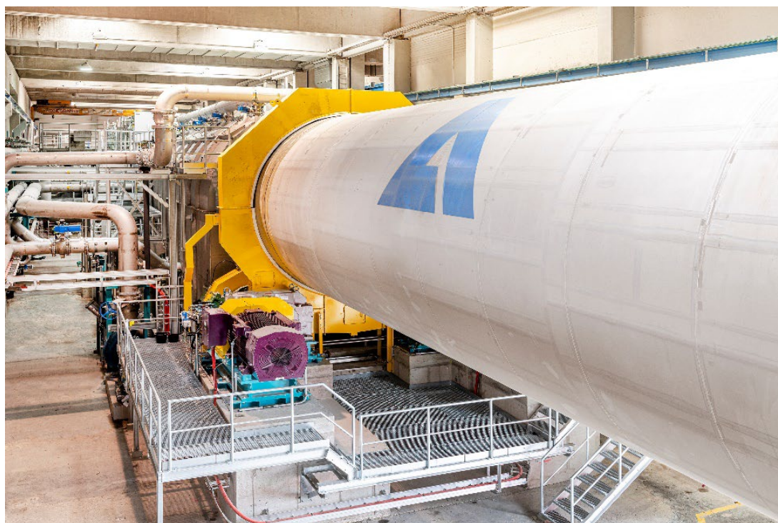
Europe's largest ANDRITZ FibreFlow drum pulper started up at Heinzelpaper Laakirchen Copyright: Heinzelpaper Laakirchen
